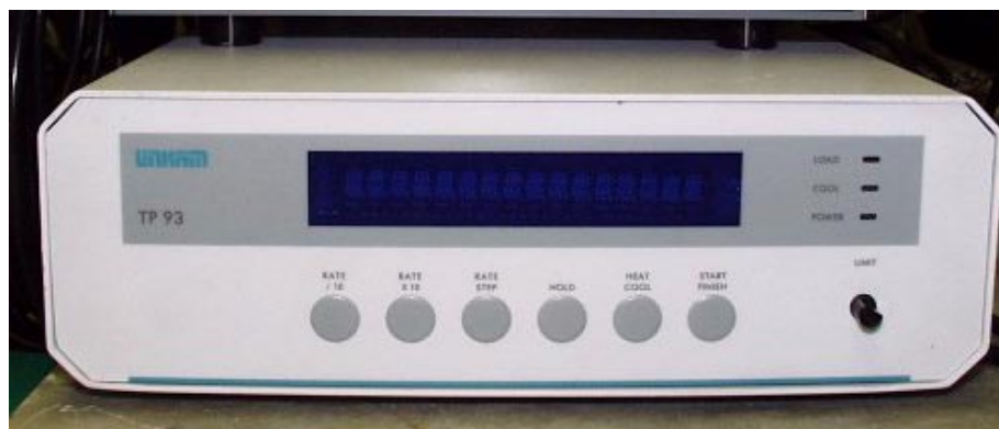
Figure 5 Temperature Stage Controller Front Panel
