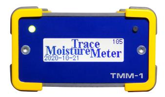
The TMM-1 Trace Moisture Meter is a universal gauge for the measurement of water in gases by the help of a phosphorus pentoxide (P<sub>2</sub>O<sub>5</sub>) electrolytic cell. Cells of most manufacturers can be used.
